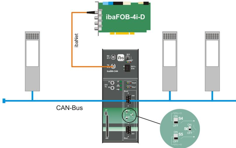
Figure 5: ibaBM-CAN connected between CAN bus devices
