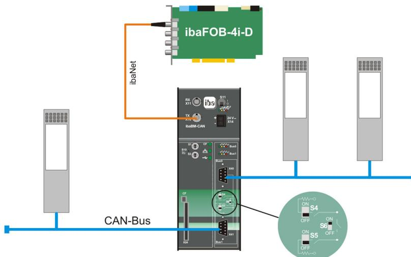
Figure 6: ibaBM-CAN in looping through mode
