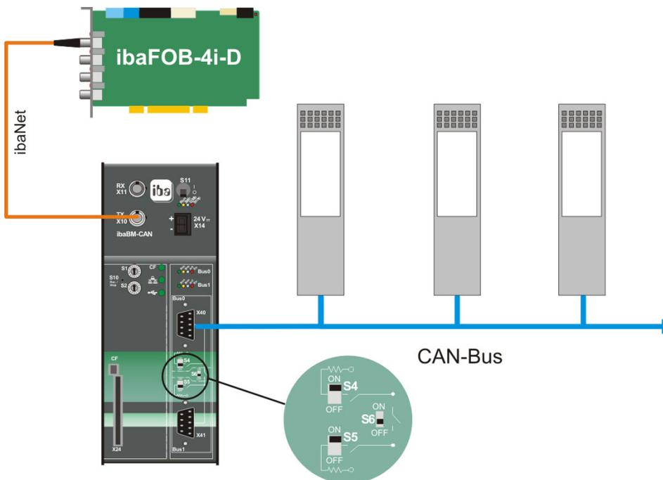
Figure 4: ibaBM-CAN connected to a CAN bus and ibaFOB-4i-D in the measuring PC
