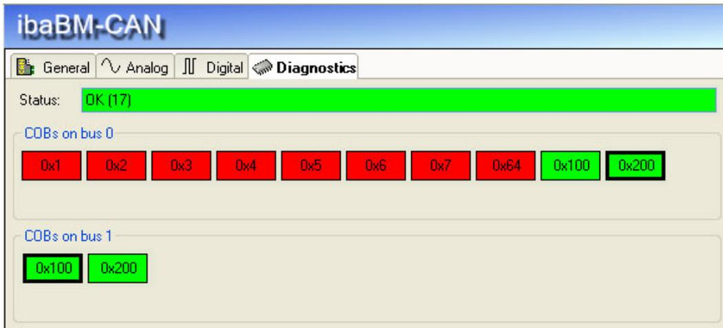
Figure 12: ibaBM-CAN – Diagnostics tab
