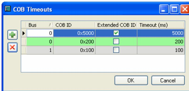
Figure 9: ibaBM-CAN, General tab – COB timeouts
